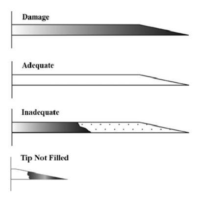
Figure E.2 – Adequate and Inadequate Crack Repair
