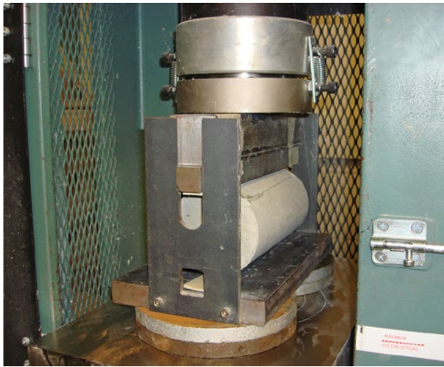
Figure 6-13. Splitting tensile strength
