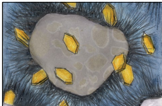
Figure 5-10. Hydration products grow during cooling
