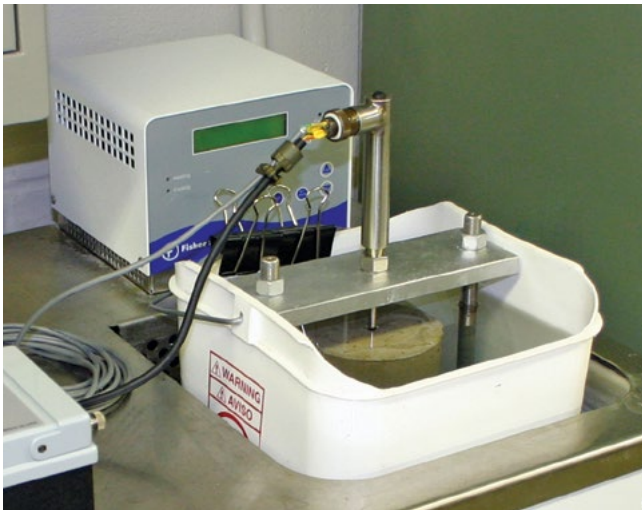
Figure 6-9. Measuring the coefficient of thermal expansion
