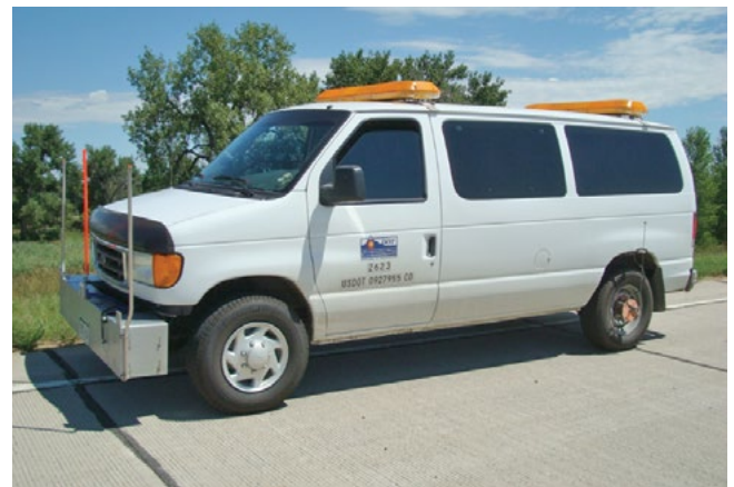
Figure 9-11. High-speed inertial profiler
