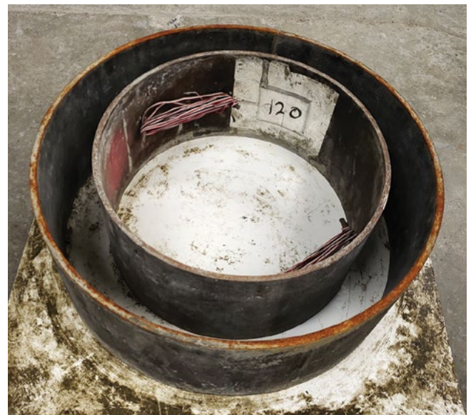
Figure 6-25. Gauged invar rings for casting concrete to monitor both expansion and shrinkage stresses
