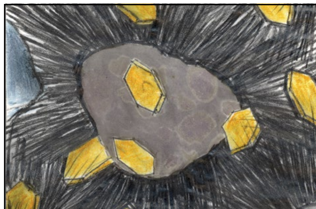
Figure 5-12. Hydration products mesh into a dense solid
