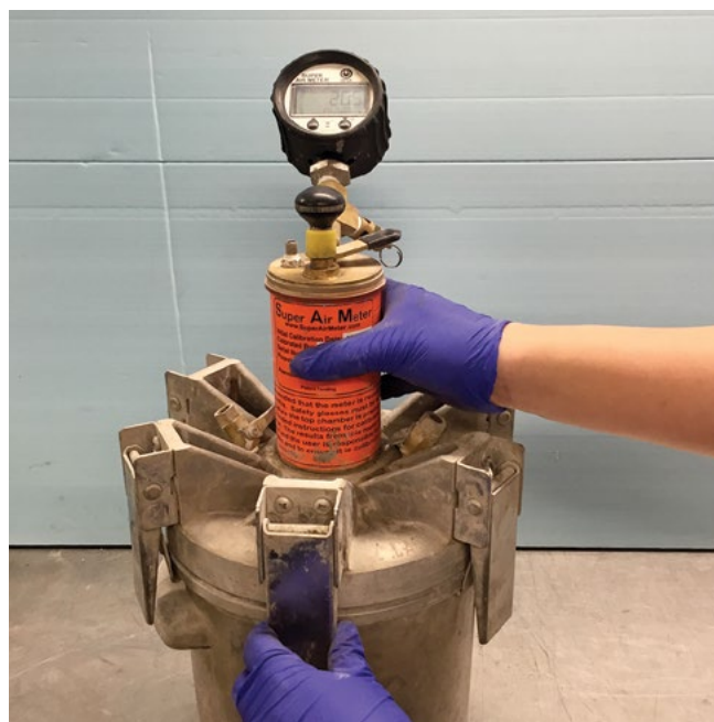
Figure 9-6. Super air meter
