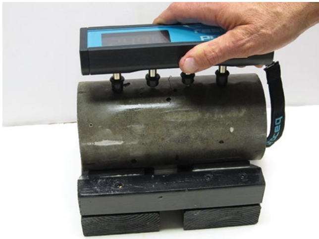
Figure 6-31. Wenner resistivity test
