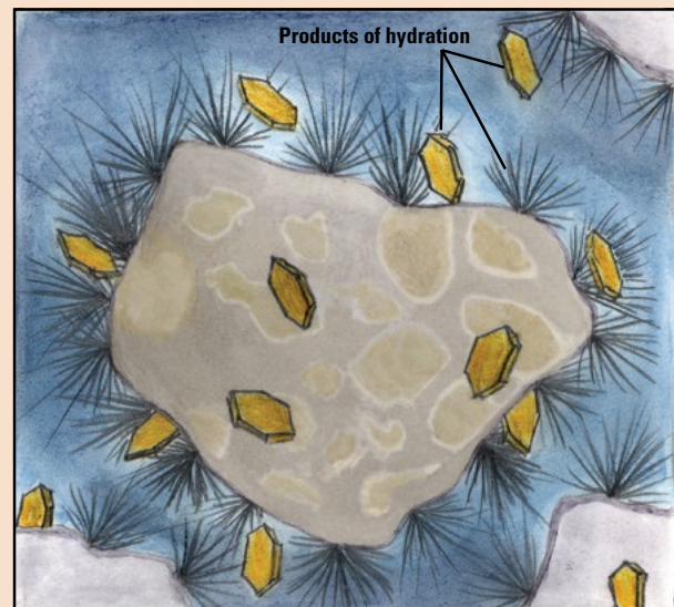
Figure 5-8. Hydration products grow
